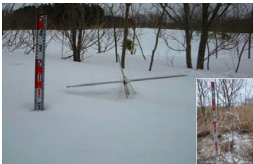
Figure 1. The multi-layer sampling unit used to estimate soil CO 2 efflux under the snowpack in at Rishiri Island, Japan. CO 2 was sampled sequentially through inlets at 120 cm, 90 cm, 60 cm, 30 cm, and 10 cm above the ground to a laboratory ~5 m away for concentration detection. The large photo shows the sampling unit in the mid-winter (February 23, 2011), while the insertion shows that before snow cover development (December 10, 2010).
